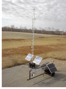
Solar Power and Fixed Cameras on a Portable Platform
